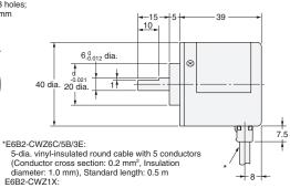
5-dia. vinyl-insulated round cable with 8 conductors (Conductor cross section: 0.2 mm², Insulation diameter: 1.0 mm), Standard length: 0.5 m
